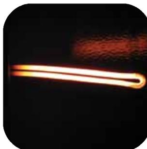
If the tank is not completely full of water when electric power is turned on, the upper element will burn out. If this happens, you'll have no hot water until the upper heating element has been replaced.
