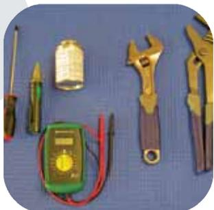
You'll need common plumbing tools and pipe joint compound (or Teflon<sup>®</sup> tape) approved for potable water. You'll also need a circuit tester or voltmeter. Most codes require the water heater to be installed in a metal drain pan. See the Installation Instructions for information about sizing the drain pan and other installation details.
